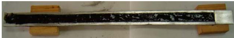
Figure 3.1: Making the MR sandwich beam: the MR fluid filling the Mid-layer cavity
