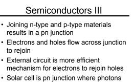
Solar cell is prijunction where protons provide energy for electrons to become free electrons
