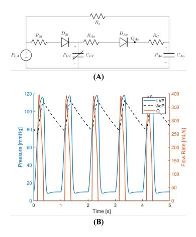
**Figure 2. (A)** Circuit representation of a normal systemic circulation and **(B)** Left ventricular pressure (LVP), aortic pressure (AoP) and aortic flow rate (Q)
