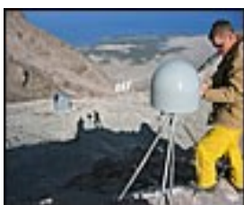
GPS receiver installation
