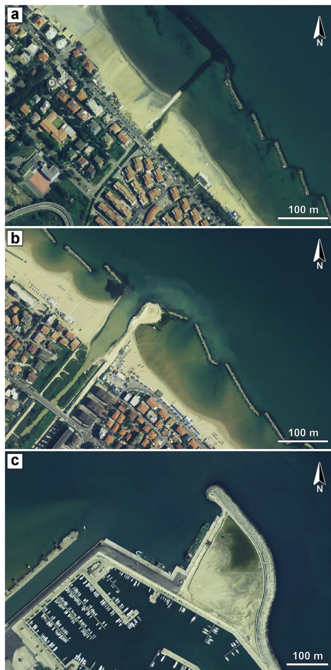
Fig. 2. Polluted water entrapped by containment cells, wharves, breakwaters, and landfill sites. Images from Google Earth 2006. Rows of containment cells extend along almost the entire 130 km length of the Abruzzo coast; (a) Containment cells formed by breakwater barriers perpendicular and parallel to the beach at the Fosso Vallelunga mouth (see Fig. 6). (b) Polluted sediments, marked by murky water from the Alento River, are dragged from rip currents within containment cells; (c) Landfill cells used to accumulate polluted sediments from the Pescara port. Pictured in 2006, the cell looks partially filled, but as of this 2017 writing it is completely filled and vegetated.
