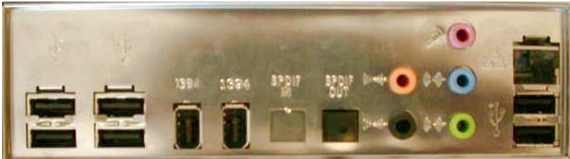
New back panel for motherboard (no ps/2, com port, printer port)
