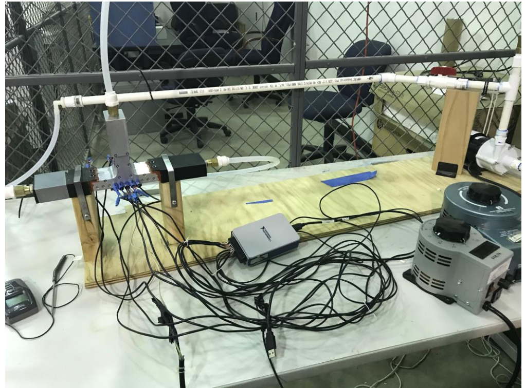
Experimental setup for liquid cooling investigations.
