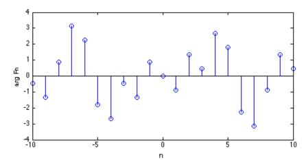
In this example, the fundamental frequency,  $f_0 = 1/T = 1/7$ . Thus, the amplitude spectrum can also be plotted versus the frequency in Hz with:
