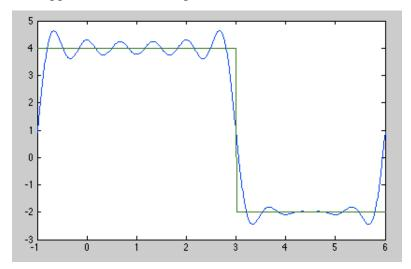
Using only seven terms the truncated Fourier series makes a reasonable approximation to the pulse train. Note that as more terms are added the approximation improves. For  $n_o = 30$ :
