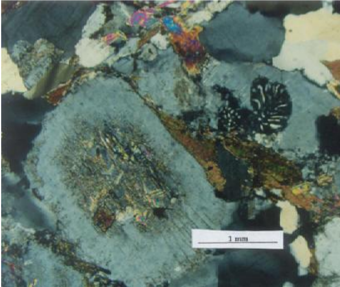
Fig. 26. Microcline (light gray) is bordered by myrmekite with very tiny quartz vermicules. Note zoned plagioclase (left side) with sericite and epidote in core. Biotite (brown).
